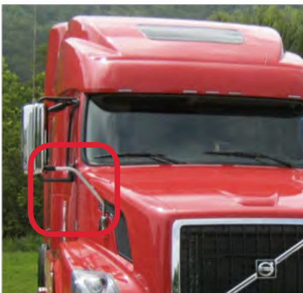
Custom kits for PACCAR and Volvo vehicles are designed for specific hood geometry and wire routing
