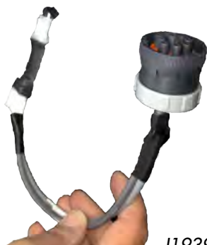
J1939 Network Provides critical engine info: idle time, fuel economy, miles traveled, etc.
