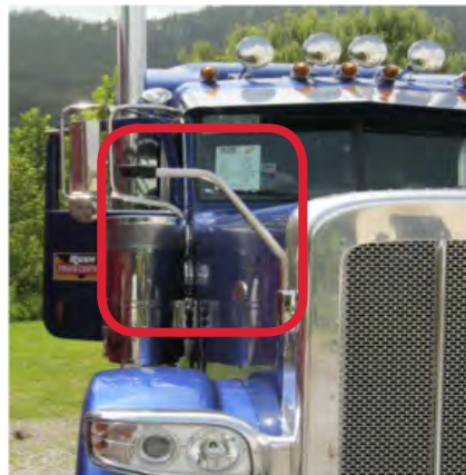
1" OD stainless steel tubing arm can be rotated for fine camera angle adjustment. Also rotates upon impact to reduce the potential damage
