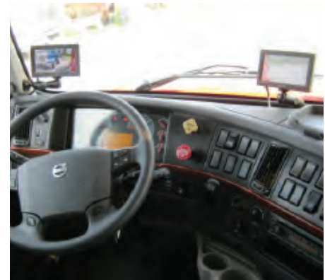
Available with right side and left side dedicated dash mounted monitors as shown above
